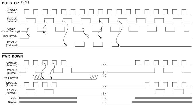
Shaded section on the VCO and Crystal waveforms indicates that the VCO and crystal oscillator are active, and there is a valid clock.
